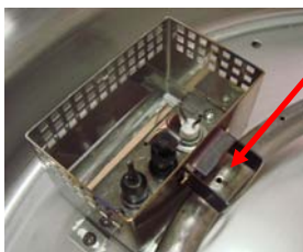
Pilot Window lined up with burner hole.
