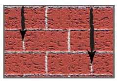
Step#6 - Conclude by painting each individual brick / tile. You can use a Left and Right pattern. Or an Up and Down pattern. Or a Swirling pattern. Lastly you may apply a fog coat to even any spotting.
