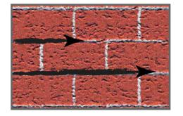
Step#5 - Follow by spray painting the brick lines in a vertical direction.
