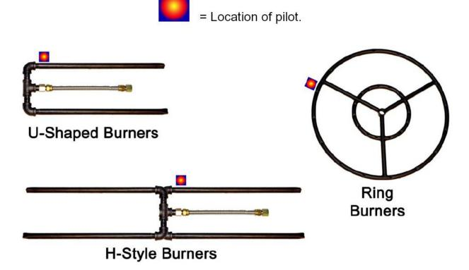
As shown above, the pilot should be as close as possible to where the gas feeds into the burner and where the gas will start coming out of the burner holes, or at a cross member location in the outer-most ring of fire rings.
